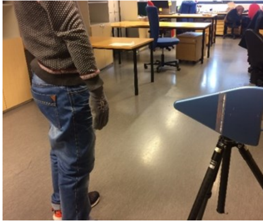
Fig. 5. Measurement setups in an anechoic room (top) and in a normal office environment (bottom), the measurement distance was 1 meter.
