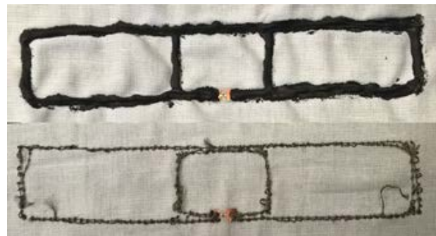
Fig. 1. Structural diagram of the studied antenna (top) and the studied UHF RFID tags made from conductive paint (middle) and conductive yarn (bottom).
