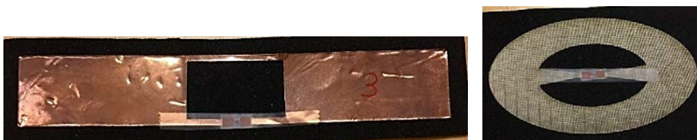
Fig. 2. Ready-made copper dipole (left) and electro-textile folded dipole (right) RFID tags.
