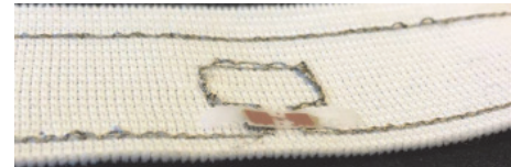
FIGURE 7: A broken glued antenna-IC interconnection.
