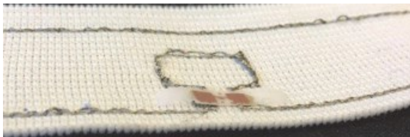
Figure 40. The broken IC interconnection [Publication II].
