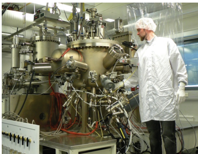
Figure 2.1. MBE grower operating a VG V90 MBE system used in the course of this thesis work. The V90 system is equipped with aluminium, indium, and gallium effusion cells as group III sources and phosphorus and arsenic crackers as group V sources.
