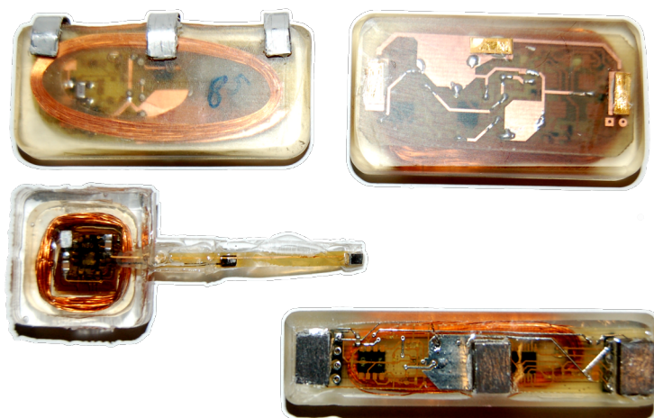
Fig. 4.3. In vivo tested implantable ECG monitoring devices realised at TUT. First prototype at the high left corner, consecutive versions running row-wise.
