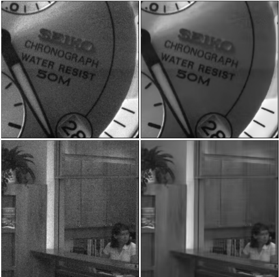
Figure C.4: Fragments of raw-data from CMOS sensor before and after Pointwise SA-DCT denoising with noise parameters estimated automatically.
