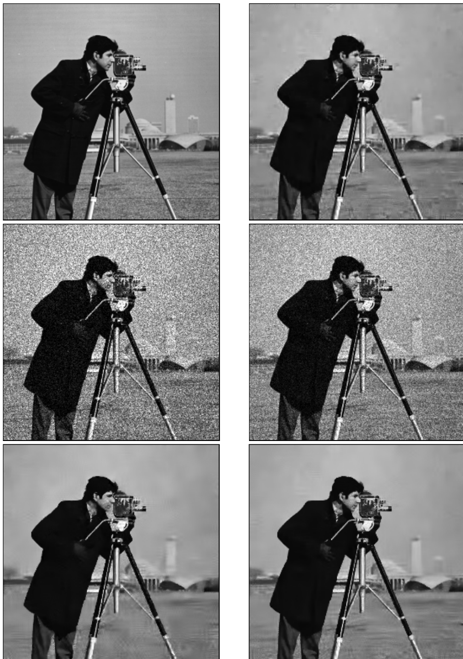
Figure 3.3: Cameraman image. Left column, from top to bottom: original image, noisy observation corrupted by Poissonian noise ( \chi = 30/255 , MSE=1015, PSNR=18.1dB), and Pointwise Shape-Adaptive DCT estimate \hat{y}^{wi} (MSE=100, PSNR=28.1dB). Right column, middle: noisy observation corrupted by Poissonian noise ( \chi = 60/255 , MSE=504, PSNR=18.1dB); top: AS B-DCT estimate [52] (MSE=70, PSNR=29.7dB); bottom: Pointwise Shape-Adaptive DCT estimate \hat{y}^{wi} (MSE=68, PSNR=29.8dB).
