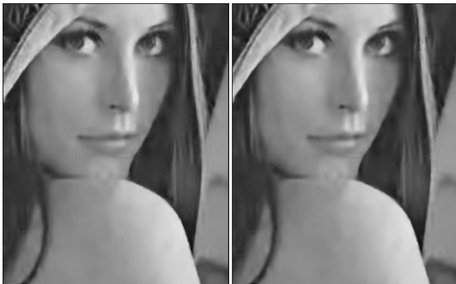
Figure 4.3: A fragment of the estimates of Lena (from the noisy observation with \sigma=25 , shown in Figure 1.10) obtained using (left) the low-complexity SA-DCT (PSNR=31.66dB) and (right) using the “shape-adapted” DCT (PSNR=31.76dB). There are almost no visible differences between the two estimates.
