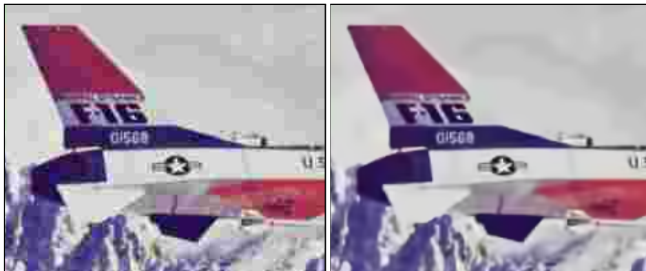
Figure 1.18: Fragments of the JPEG-compressed ( Q=10 , 0.25bpp, PSNR=26.87dB), and restored F-16 color image (PSNR=28.30dB) using the proposed Pointwise SA-DCT deblocking filter in luminance-chrominance space.
