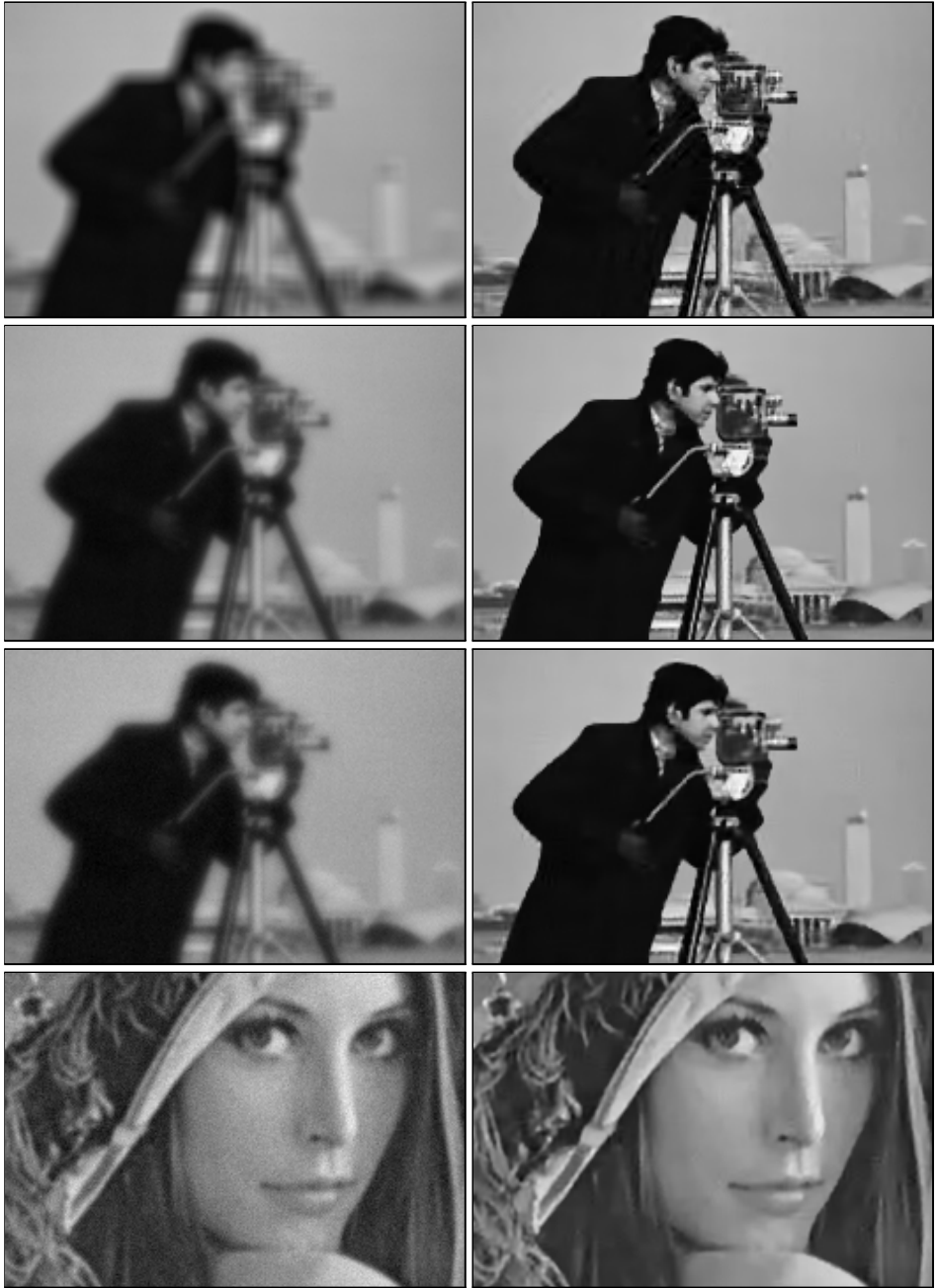
Figure 2.8: From top to bottom: fragments of the observations z and of the corresponding Pointwise SA-DCT estimates \hat{y}^{RWI} of four deblurring experiments. The ISNRs of these estimates are 8.57, 8.25, 6.34 and 4.52 dB, respectively.
