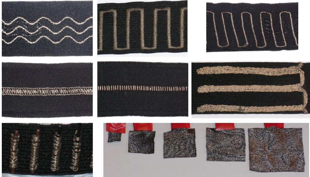
Figure 20. A sample of electrode surface structures used in the experiments. The electrode squares used in the studies leading up to Papers 2, 3, and 4 were cut from the textile sheet shown in the bottom right hand corner. For size comparison, the elastic ribbons used for the embroideries had a width of 3 to 4 cm.
