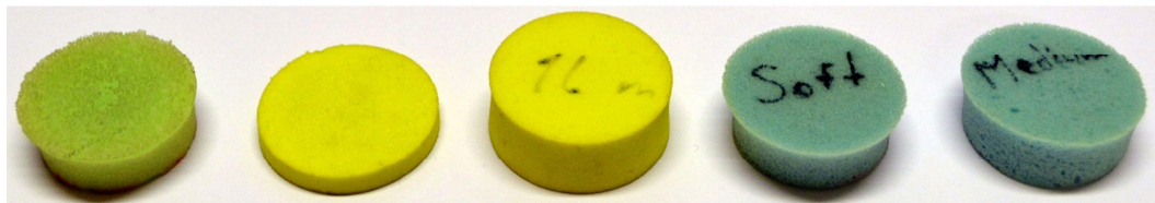
Figure 21. The paddings used between garment and electrode in Paper 1. The radii of the paddings are between 16 and 19 cm, and the thickness from 6 to 16 mm.
