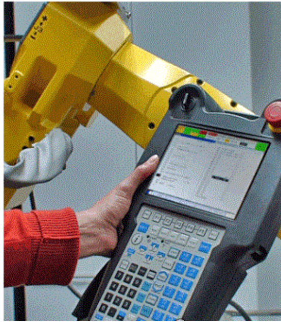
Figure 1. A teach pendant used in online programming (Motion Control Robotics 2017)
