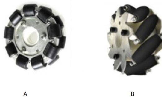
Figure 1. Two types of omnidirectional wheels, A) a omni wheel, B) a mecanum wheel [2]
