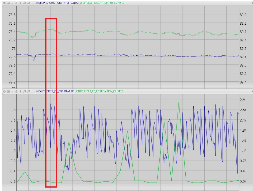
Figure 37. Correlation analysis for the first and last causticizing chamber CE-% difference. The time point with the strongest correlation is used to determine the signal time delay shift.
