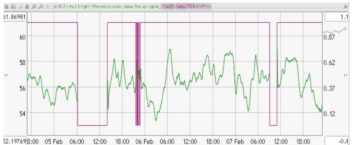
Figure 14. Validated process data. A quality based process control is usually evaluated by the decrease of normal operation variation. Data validation can mean a decrease of tens of percentages in variation, thus evidencing the importance of defining the right set of data.
