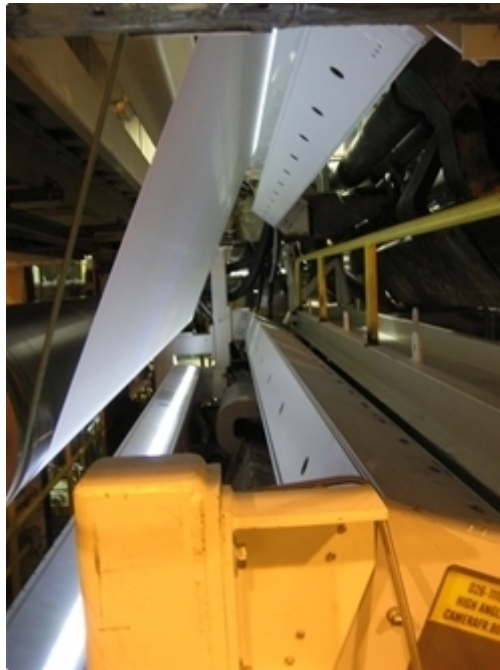
Figure 6.2. Metso PQV web inspection system integrated into paper machine.
