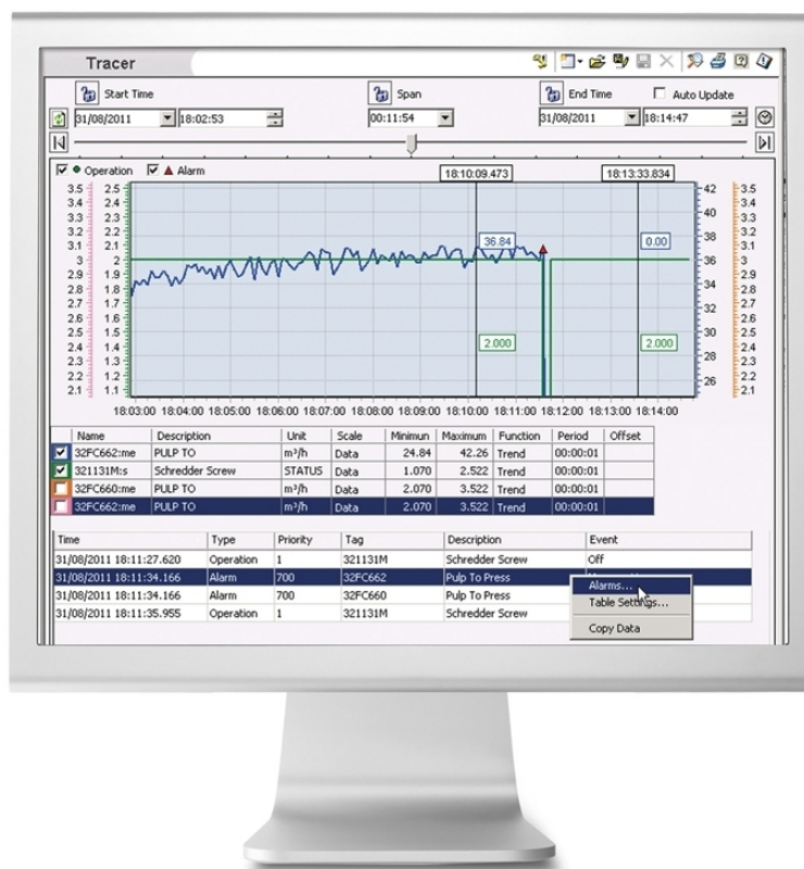
Figure 6.4. Metso DNA Tracer automatically combines trends, alarms, operations, messages and diary entries of the selected tags in the same picture.
