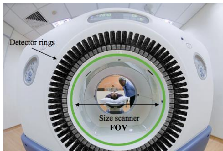
Figure 2.5. Position of detector rings and scanner FOV for a PET device.
