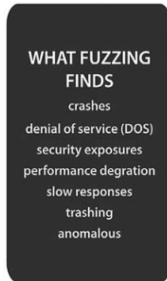
Figure 3.2 Fuzz testing can cause the underlying SUT to different failure modes. Figure modified from [66].
