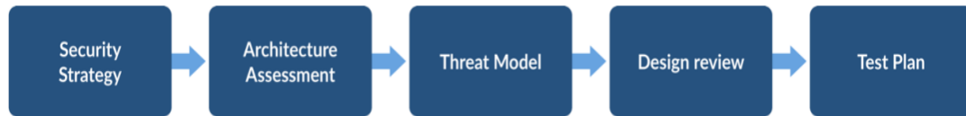
Figure 2.6 Threat modeling is performed after architecture of the system is reviewed and it guides the following test plan [35].
