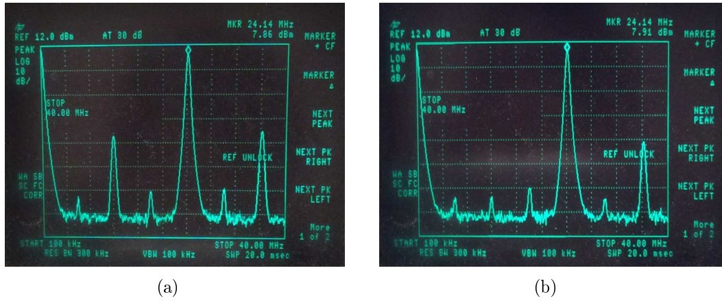
Figure 4.10 (a) The spectrum of XO working without buffer and (b) the spectrum of XO working with buffer.
