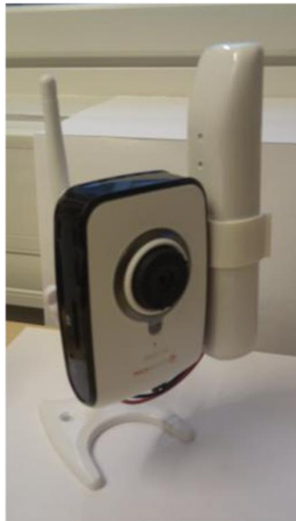
Figure 5.1: A working prototype has a WLAN camera and a low-power TUTWSN node for camera wakeup.
