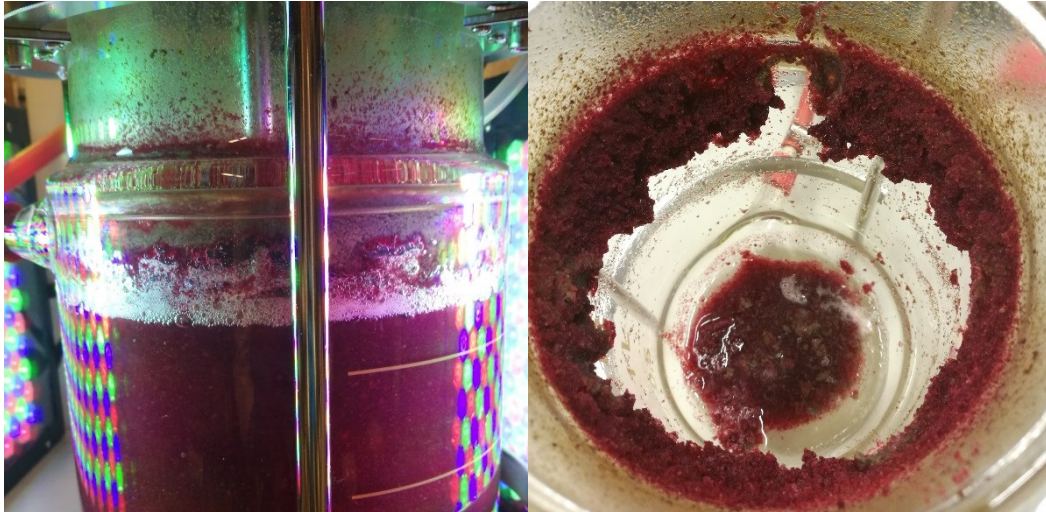
Figure 23. Lingonberry-6 batch with foaming and cell growth problem. The left picture was taken at the end of cultivation, before emptying the bioreactor. Grey areas of dead cells can be seen in the middle of the attached cell layer. The right picture was taken before washing the bioreactor to illustrate the amount of attached cells.
