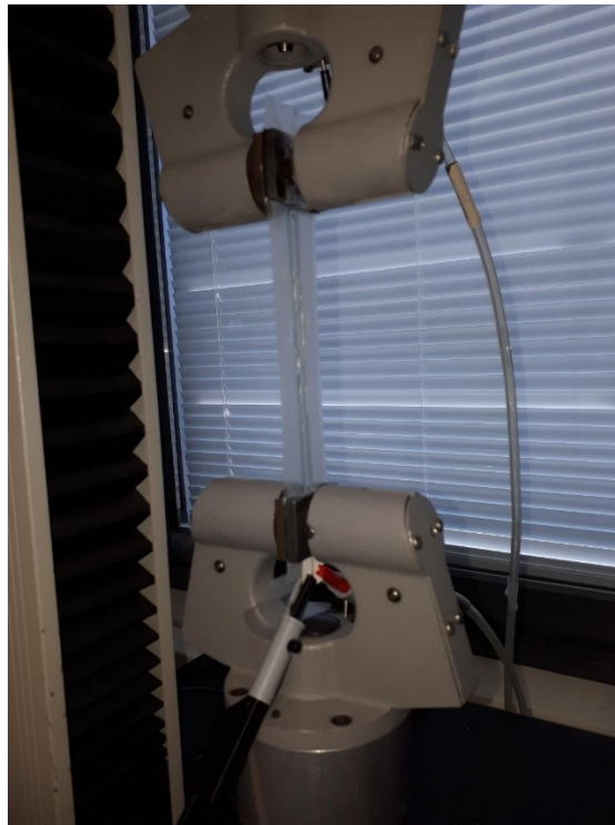
Figure 35. A transfer tattoo mounted to Instron 4411 for electromechanical and mechanical testing.
