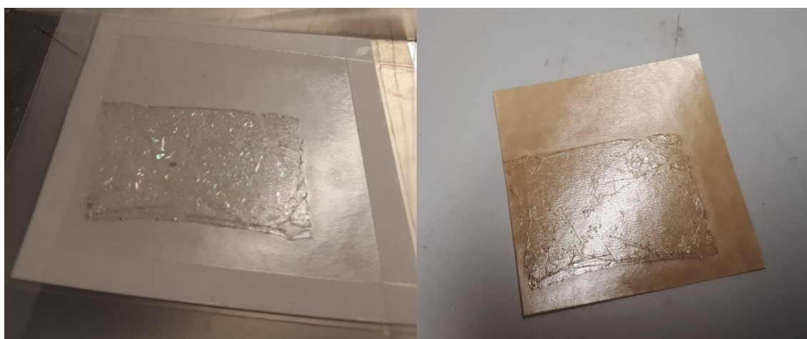
Figure 28. The tattoo paper before (on the left) and after (on the right) removing wrinkles from the PMMA film in an oven.
