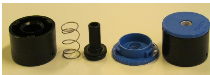
Figure 4 – The assembled cylinder and its components
