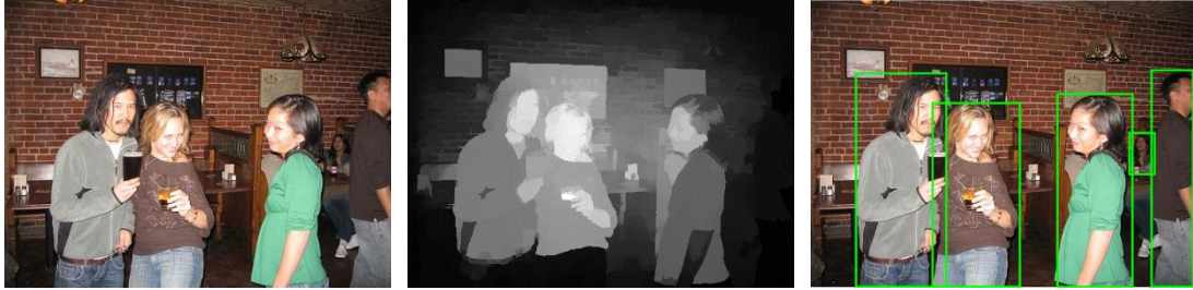
Figure 22. Not all objects are salient: (from left to right) Original Image, Saliency Map, Object Proposal ground truth (green)
