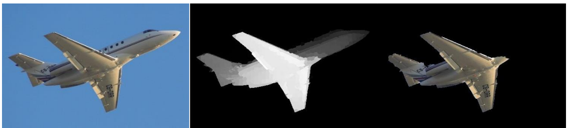
Figure 24. Proposal extraction using Adaptive Thresholding on Saliency Maps: (from left to right) Original Image, Saliency Map, Proposal extracted through adaptive thresholding
