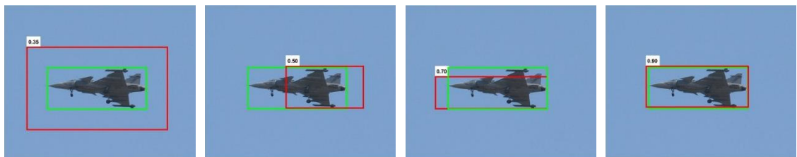
Figure 32. IoU Overlap: (from left to right) IoU Overlap of 0.35, 0.50, 0.70 and 0.90 respectively between green and red proposals
