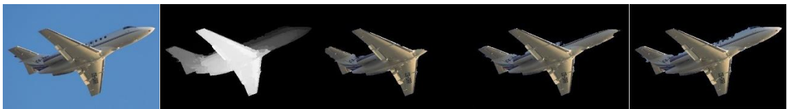
Figure 25. Multi-level thresholding based proposal extraction: (from left to right) Original Image, Saliency Map, Proposals generated through multilevel thresholding
