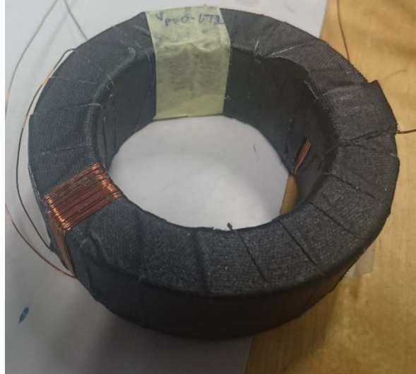
Figure 5.6: The prototype of nanocrystalline core.
