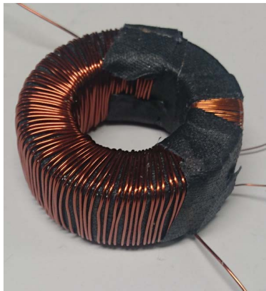
Figure 5.3: The prototype of 2605SA1 amorphous core.
