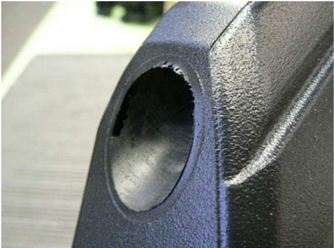
Figure 8. Example of burr formed on a parting line between mould segments.
