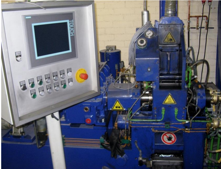
Figure 4.1. Intermeshing mixer used for compounding rubbers
