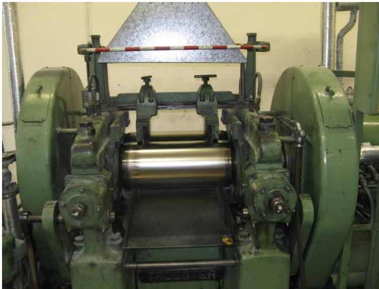
Figure 4.2. Two roll mill used for compounding rubbers
