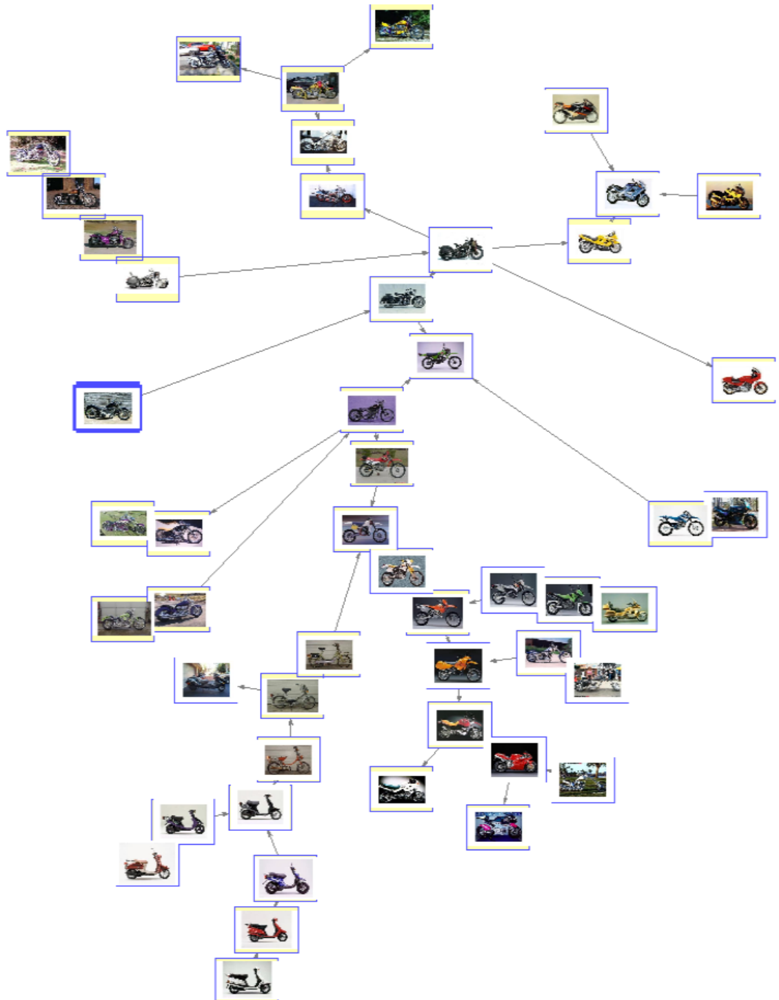
Figure 26. Minimum spanning tree created for the graph in Fig. 25. Root (seed) is specified with dark blue border. Note that images with less similarity to the seed are located far from the root. Also, images with the same intra-class type such as scooters are arranged in a same branch.
