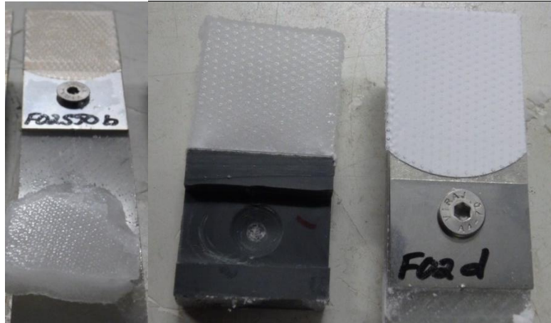
Figure 45. Supplier M2's membrane of 0.2 \mu\text{m} pore size had a supporting matrix behind the structure. This resulted in the same texture to accreted ice pieces contacting the PTFE –membrane. The texture was seen in both, lubricant infused samples and in plain membrane samples which had no lubricant impregnated into.
