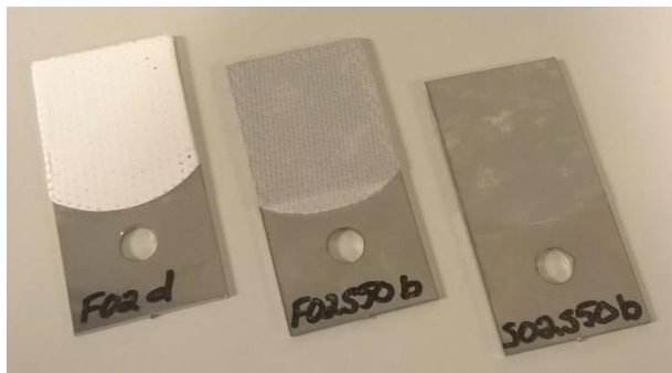
Figure 31. The unmasked SLIPS samples on a metallic substrate ready for masking and cyclic icing test.
