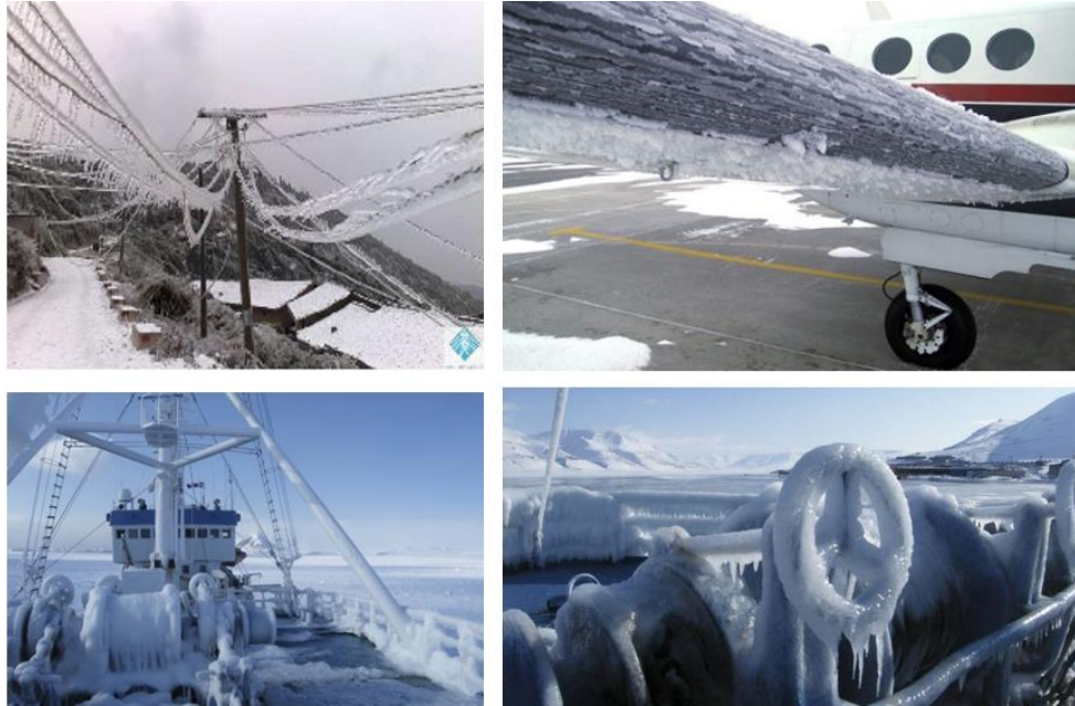
Figure 23. Different icing problems caused by ice accretion on different systems from cables and airplanes to maritime vessels. (DNV GL AS, 2015; Mastenbroek Aeroskill, 2015; SWZ Maritime, 2014; Yinhe Wind Power Co. Ltd., 2012)
