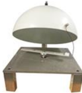
Figure 33. The centrifugal ice adhesion test machine with a sample to be tested inside.
