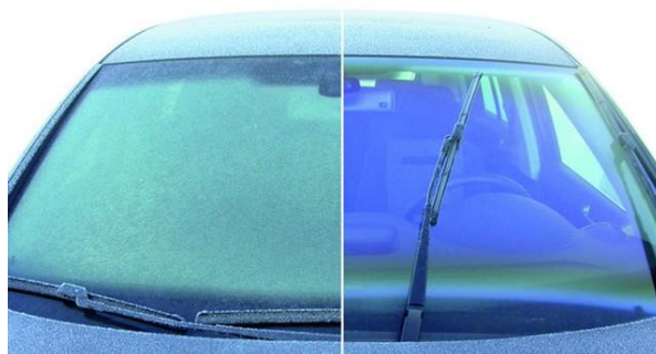
Figure 10. By examining and studying different coating solutions, even frost-free windshields are made possible. A coating of indium tin oxide has been applied on glass by Volkswagen. (Tokic, 2015)
