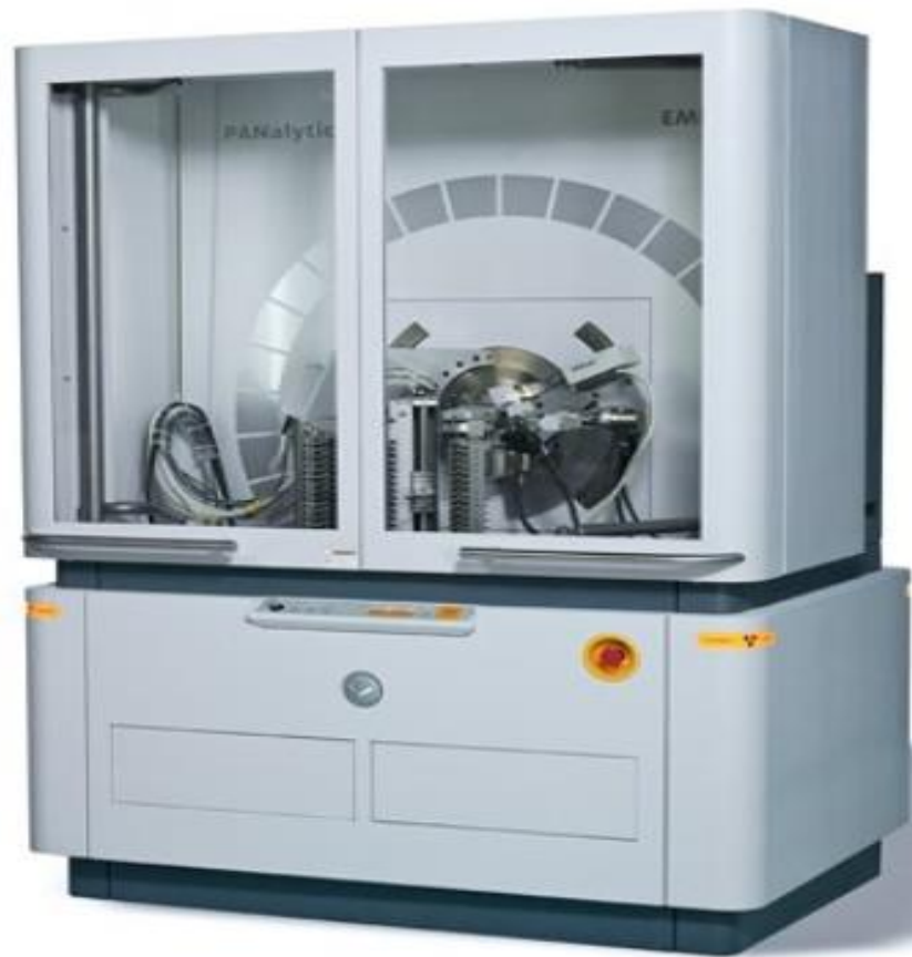
Figure 32 b. General schematic illustration of Panalytical Empyrean Multipurpose Diffractometer equipment, which is used to analyze the XRD pattern of deposited thin films. [117]
