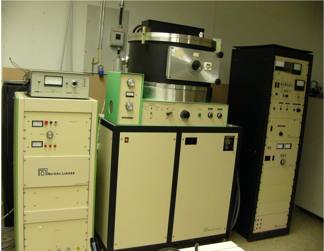
Figure 23. Overall representation of Nordiko NS-2500 sputtering equipment used in this research work with RF (Radio-frequency) power supply unit and control units is shown in this Figure.
