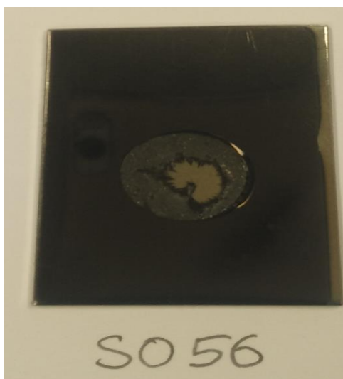
Figure 67. Adhesion tested surface of sputtered titanium nitride coating using adhesion p.a.t.t.i equipment is presented in this Figure. The sample S056 used for adhesion test are sputter etched for 10 minutes with 100W RF power. The deposition parameters used for S056 is given as follows current – 2 A, deposition time - 10 minutes, argon sputtering pressure – 5 mtorr and nitrogen sputtering pressure – 2 mtorr.
