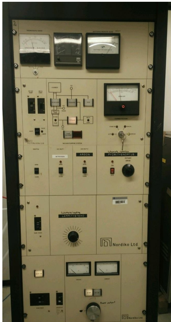
Figure 29: Control unit of Nordiko NS-2500 sputtering equipment, which acts as a main operating mode of functioning the sputtering equipment efficiently with power supply units and also controlling the vacuum created in sputtering system.
