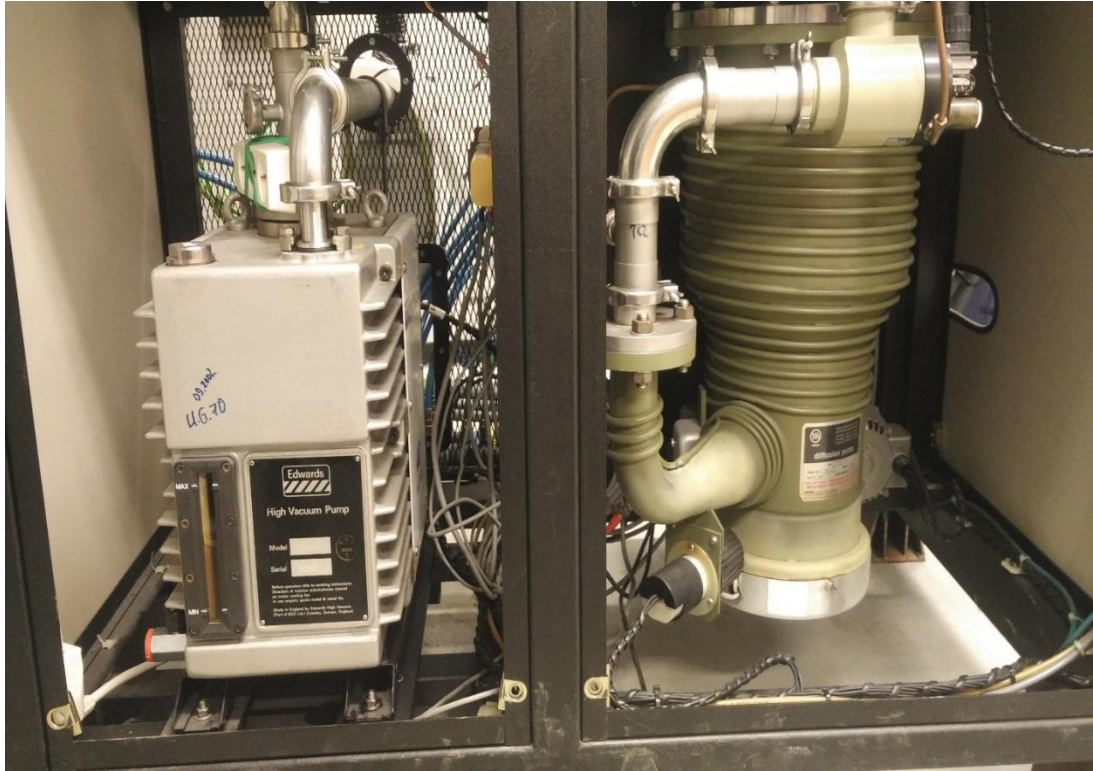
Figure 24: Typical representation of the mechanical pumps (left) and foreline pump (right) used in this Nordiko sputtering equipment is presented in this Figure.
