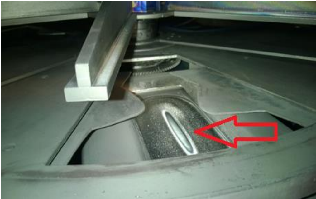
Figure 5. “Racetrack” present in our planar magnetron sputtering target material. The arrow marked in the Figure represents the path of sputtering process, following the confined path of magnetrons used.
