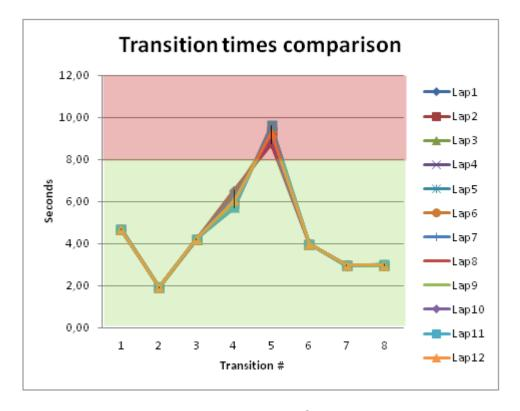
Figure 48: Flaw detected on the 5<sup>th</sup> transition of the pallet
