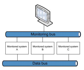
Figure 3: Generic single process-monitor architecture [Goodloe & Pike 10]
