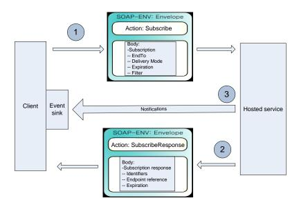
Figure 15: DPWS subscription mechanism
