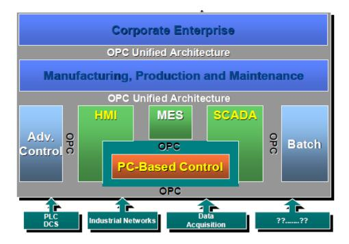
Figure 17: OPC-UA interaction in the automation levels [Burke 06]
