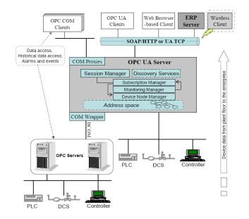
Figure 22: Architecture for monitoring and controlling of field devices [Van Tan et al. 09]
