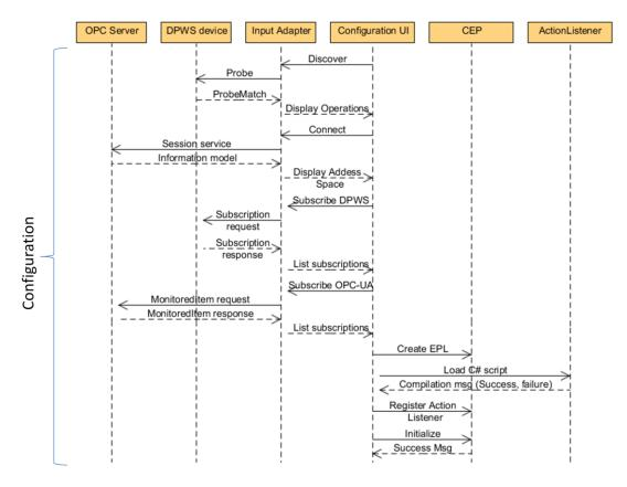
Figure 41: Deployment and configuration model
