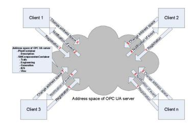
Figure 21: Interaction of clients with the address space [Schleipen 08]
