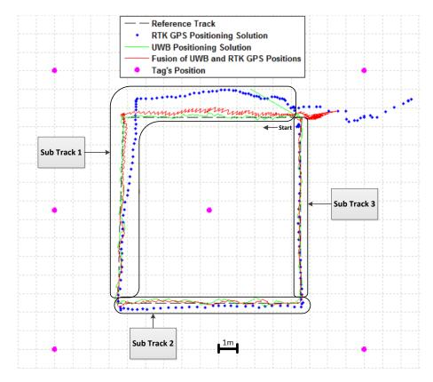
Figure 4.2. Track is divided into three sub tracks.
