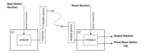
Figure 2.16. RTK GPS configuration through internet.
