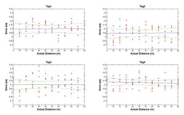
*Figure 2.8. Static line-of-sight error measurement (red \*), linear regression line (continuous blue line) and 95% credibility interval limits (green dashed line).*
