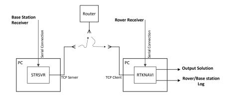
Figure 2.18. RTK GPS configuration used in thesis.
