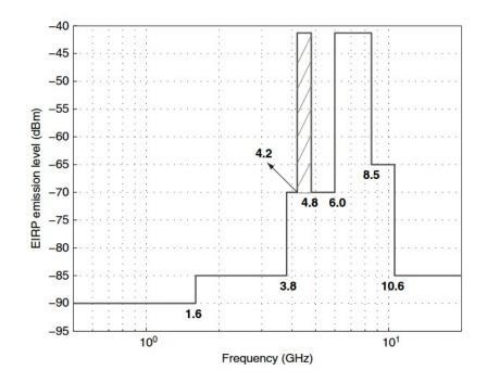
*Figure 2.4. ECC EIRP emission limits for UWB system without appropriate mitigation techniques*[1].
