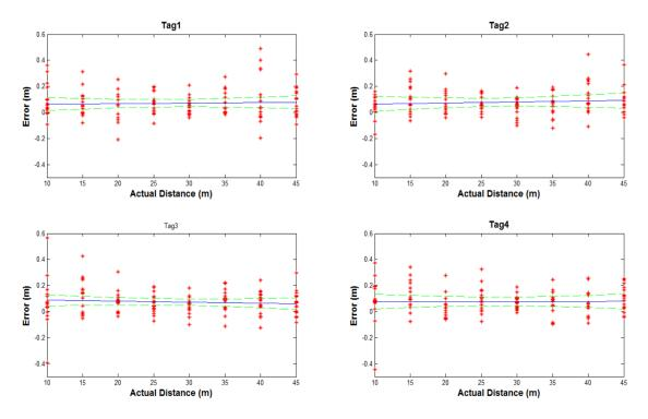
*Figure 2.9.* Dynamic line-of-sight error measurement (red \*), linear regression line (continuous blue line) and 95% credibility interval limits (green dashed line).
