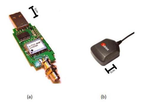
Figure 2.10. (a) Yuan10 USB receiver (b) ANN-MS u-blox active GPS antenna
