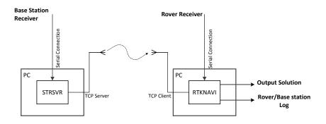
Figure 2.15. RTK GPS configuration through WiFi.
