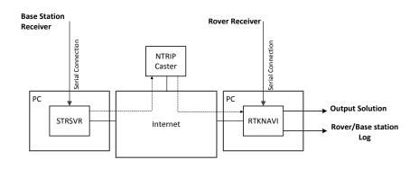
Figure 2.17. RTK GPS configuration through NTRIP Caster.
