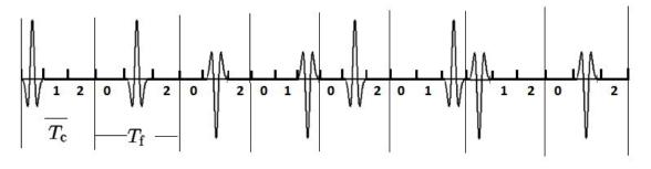
Figure 2.3. 4 bits 1010 transmission through UWB signal.
