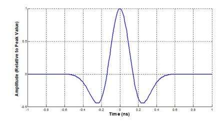
Figure 2.2. UWB example pulse shape.
