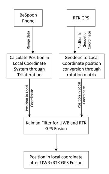
Figure 3.4. RTK GPS + UWB fusion process flow.
