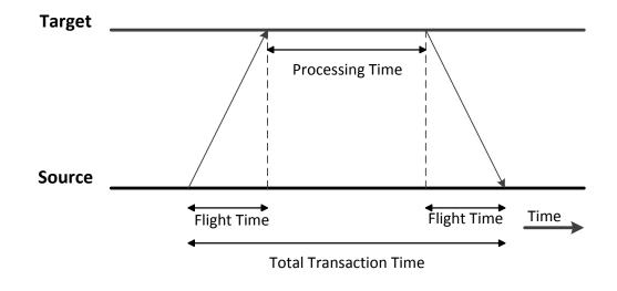
Figure 2.6. Ranging through two-way time-of-flight method.
