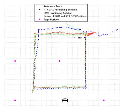
Figure 4.4. Result with four UWB tags second scenario.
