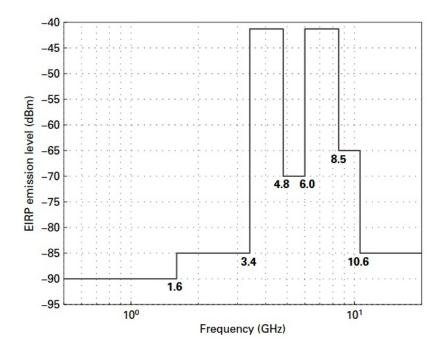
*Figure 2.5.* ECC EIRP emission limits for UWB system with appropriate mitigation techniques[1].
