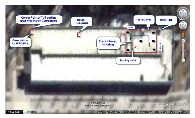
*Figure 3.7. Google Earth view of testing setup. Parking is approximately 100m long and 30m wide.*
