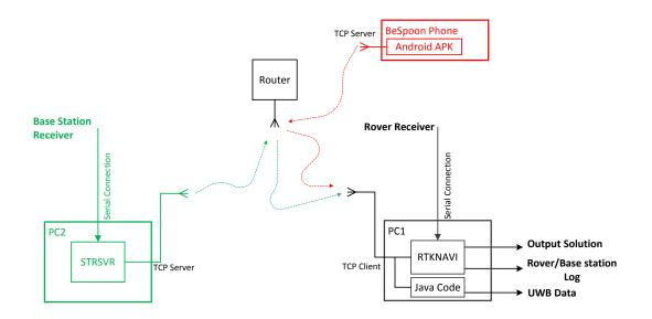
Figure 3.2. UWB and RTK GPS fusion configuration in our measurements.
