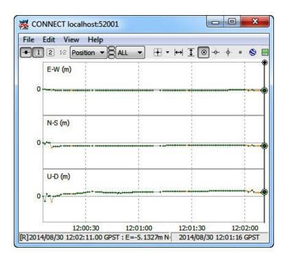
Figure 2.19. Sample testing result of RTK GPS positioning.
