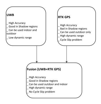
Figure 3.1. UWB and RTK GPS fusion properties.
