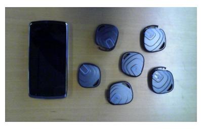
Figure 2.7. BeSpoon phone and six tags equipped with UWB.
