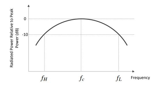
Figure 2.1. UWB signal definition.
