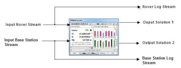
Figure 2.13. RTKNAVI data flow.
