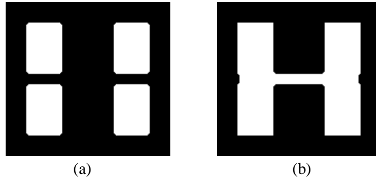
Figure 2.4: Opening and Closing. Result of (a) opening and (b) closing on the test image of Figure 2.1.
