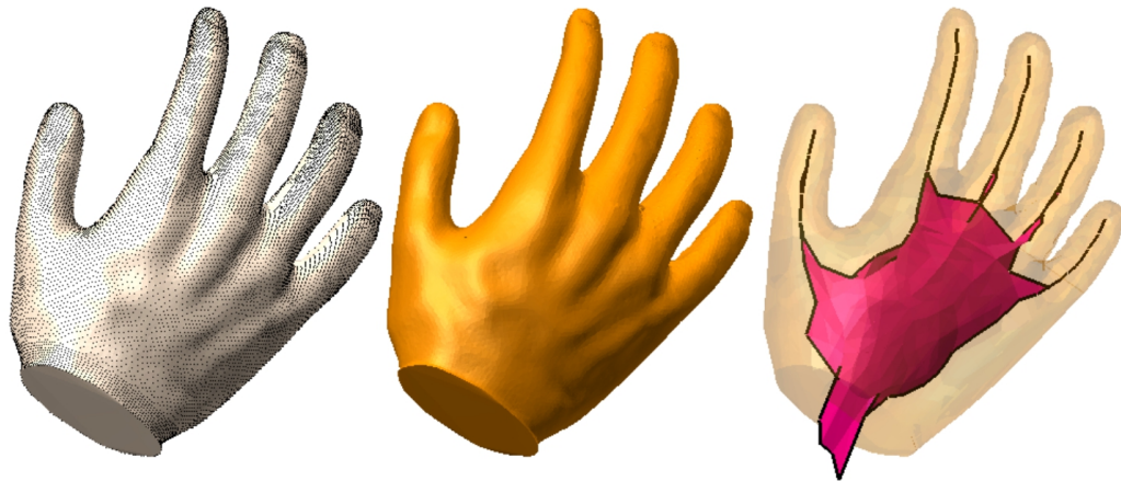
Figure 26: Point set on the left, model produced by power crust in the middle and the approximated medial axis on the right [41].
