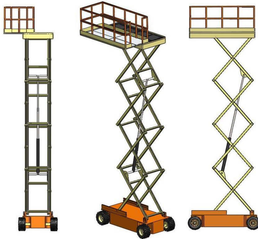
Figure 4.20. The updated mechanical structure of the MEWP.
