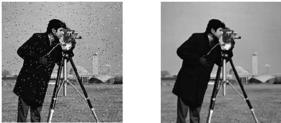
Figure 10. Left, Image corrupted with salt and pepper noise. Right, Corrupted image after median filter.
