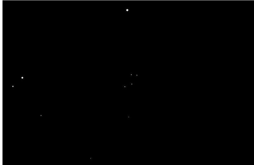
Figure 13. Image segmented, bright spot on top is another camera, and the constellation is in the middle.
