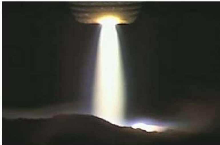
Figure 12. Stable arc in DC furnace [14]
