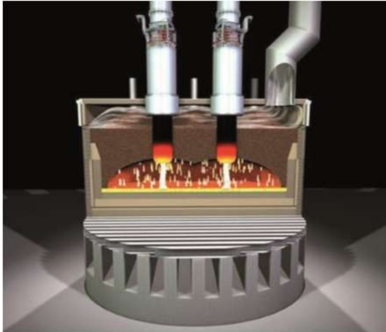
Figure 5. Modern AC-furnace in ferroalloys application [18]
