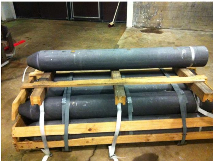
Figure 16. Prebaked graphite electrodes
