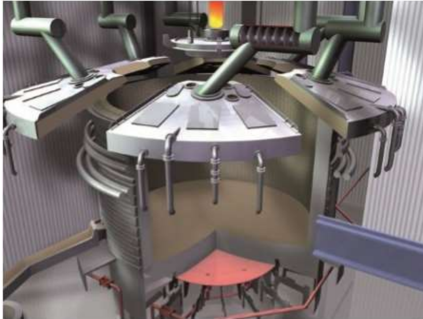
Figure 2. Modern DC-furnace by SMS-Siemag [18]
