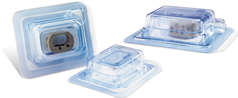
Figure 18. Double trays with an inner and outer tray for double sterile barrier packaging of spinal implant products by Orthofix. The material is PETG sealed with coated Tyvek®.
