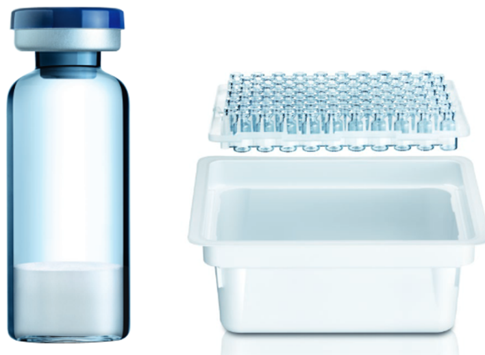
Figure 12. Left: A SCHOTT TopLyo® Type 1 glass vial with a hydrophobic coating, designed specifically for a lyophilisation process. Right: Vials can be packaged in a nest, which is then placed in a tub. Schott covers the tub with a Tyvek® inlay, and also seals it by a Tyvek® seal. The tub is further packed in a header bag and sterilized.
