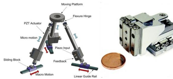
Figure 2.2 3-PUU parallel micromanipulator (University of Macau, China) [20]; 3DOF Serial micromanipulator (SmarAct GmbH, Germany) [21].
