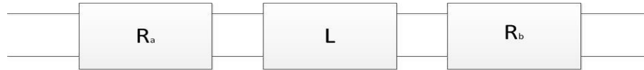
Figure 3.3. Transmission line consisting of two error boxes R_a , R_b and a central length of L .
