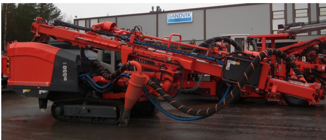
Figure 4: New DI550 DTH-rig.
