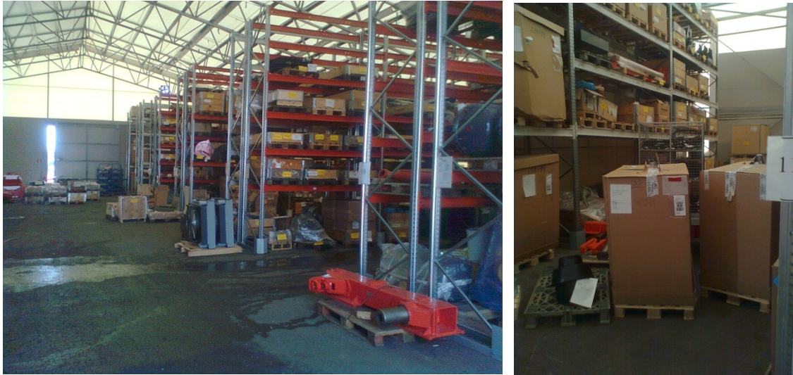
Figure 11: Pallet shelves on the SF side in MP1 storage tent. Outdoor forklifts do not fit to operate on isles and items are therefore left on isles.
