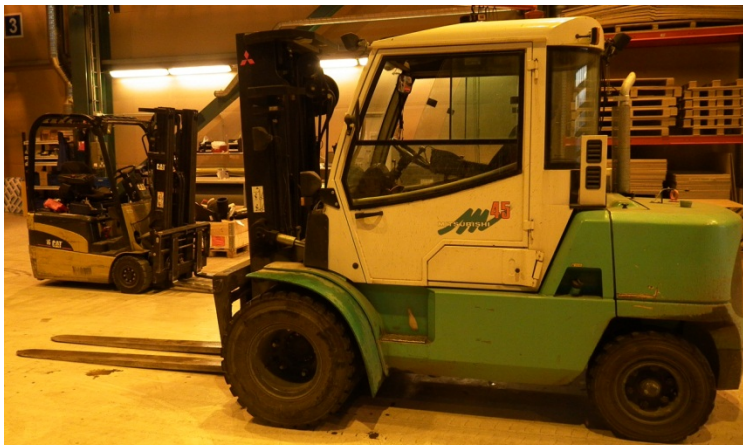
Figure 10: Forklifts used; 4,5t outdoor diesel forklift in front and 1,6t indoor electric forklift further back.
