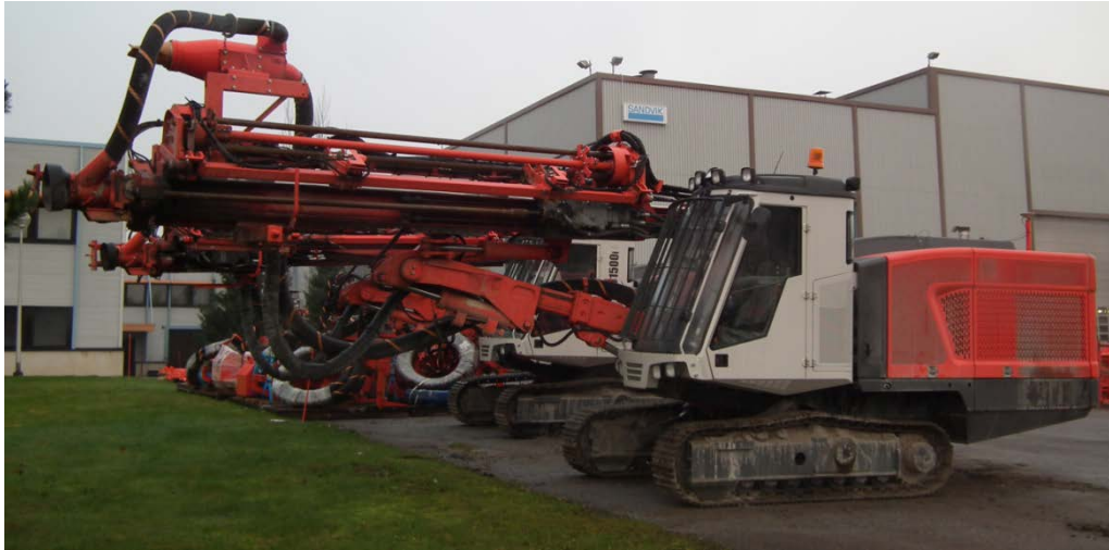
Figure 2: Slightly dirty after test drilling, DPi-series top hammer drill rig in front of MP3 building.
