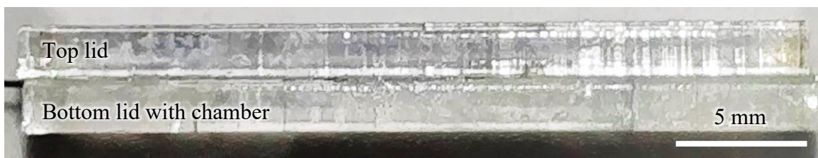
Figure 4.6. PMMA chip sideview. Top lid and bottom microfluidic structure bonded by using a thin layer of ethanol between both lid and channel for 15 minutes in an oven at a temperature of 68 °C.
