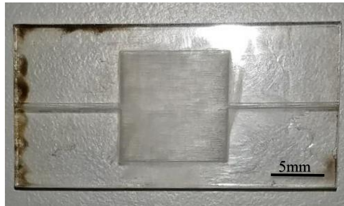
Figure 4.5. Laser engraved PMMA microfluidic chip.
