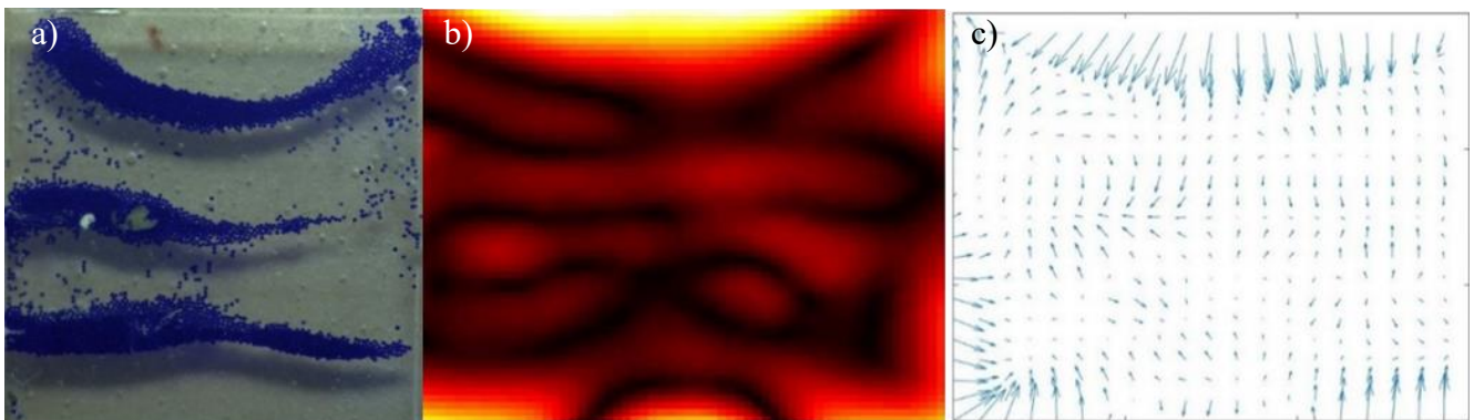
Figure 5.11. a) Acoustic pattern obtained at frequency 138 kHz, b) heatmap of the magnitude of particle mobility captured via PTV (black color denotes pressure nodes and red-yellow color denotes pressure antinodes), and c) quiver plot of PTV data.
