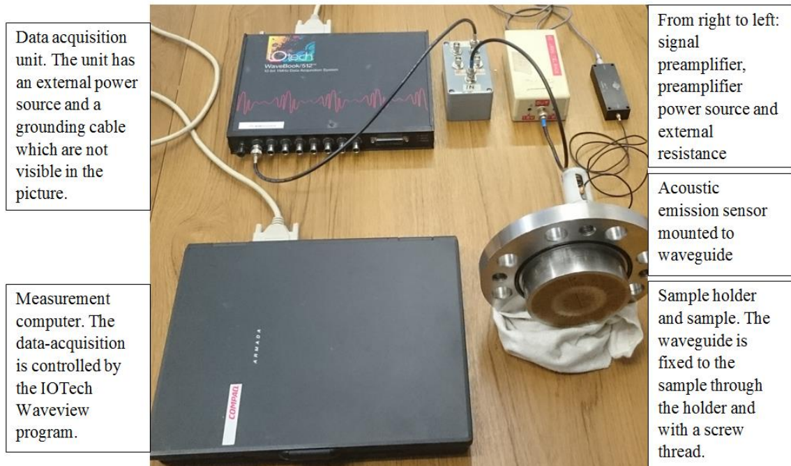
Figure 4.5. Acoustic emission measurement setup with the sample and the sample holder.
