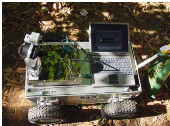
Fig.5. Mobile robot with sonar scanner [21].
