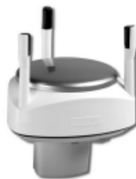
Fig.10. Vaisala WINDCAP ultrasonic wind sensor [33].
