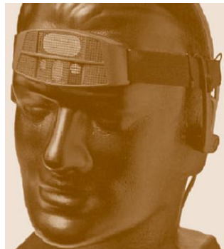
Fig.16 . Aid for blind people. Oval shaped is transmitter and the other three are receiver [3].
