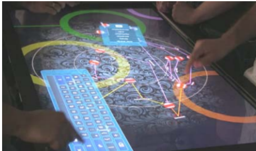
Figure 2.2 Tabletop concept mapping, tracking individual participation on the tabletop. Visualisations for longitudinal participation, contribution and progress of a collaborative task at the tabletop. Roberto Martinez [28]
