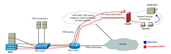
Figure 5.1: A translated connection is blocked by a firewall.
