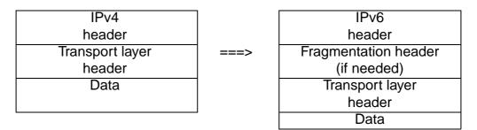
Figure 3.1: Stateless IPv4 to IPv6 translation. [RFC6145, Section 4, Figure 2]
