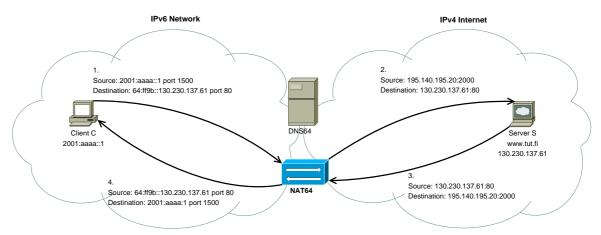
Figure 3.11: A connection between an IPv6-only client and an IPv4-only server.
