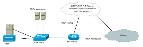
Figure 4.2: Network topology of the test setup for DNS64/NAT64.
