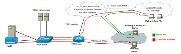
Figure 4.5: The two possible routes to the Internet from the test PC's.
