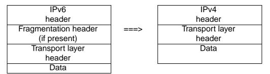
Figure 3.8: Stateless IPv6 to IPv4 translation. [RFC6145, Section 5, Figure 5]
