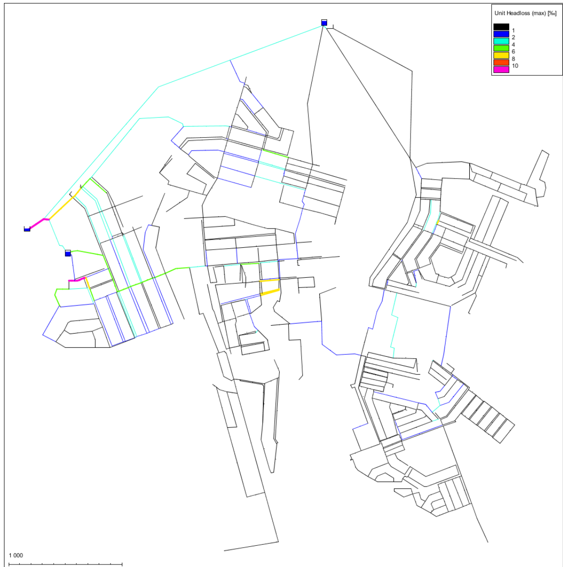
Fig. 5-15. Maximum unit head loss in Keetmanshoop's WDN [%].
