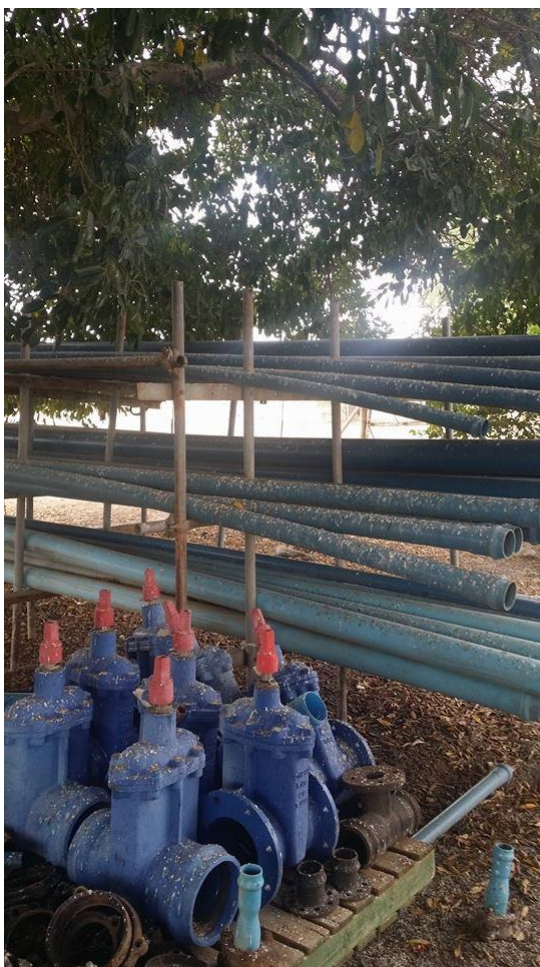
Fig. 6-1. Storage of uPVC pipes and gate valves at the municipality's warehouse (Salmivirta 2015).
