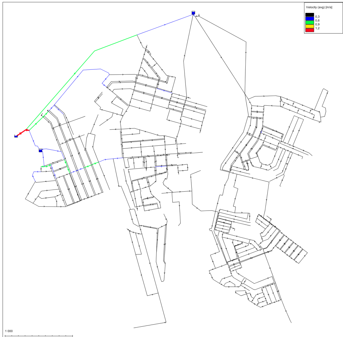
Fig. 5-16. Average flow velocity in Keetmanshoop's WDN [m/s].
