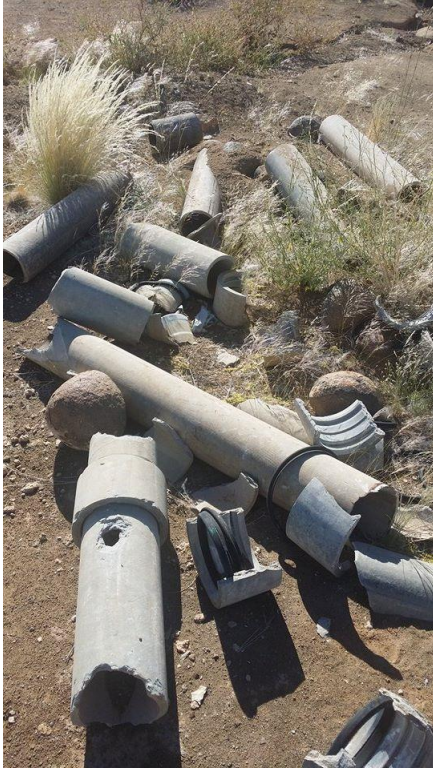
Fig. 5-1. Old AC pipes left at site after disposal (Salmivirta 2015).
