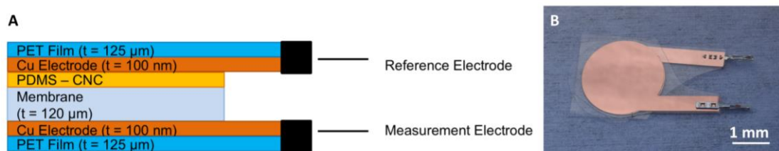
Figure 10. Sensor design for piezoelectric measurements of PDMS-CNC composite membranes. Schematic drawing (A) and photograph (B) of the sensor set-up. (Adapted from [115])
