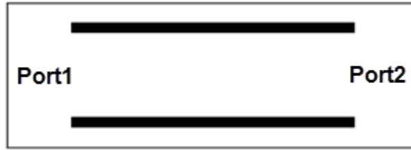
Figure 3.5 Four port differential DUT model
