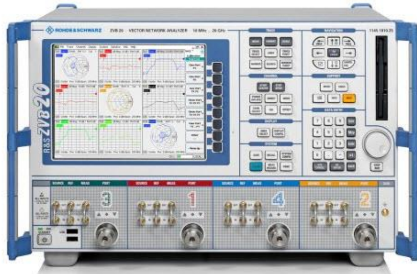
Figure 5.4 Roche&Swarz Vector Network Analyzer [26]
