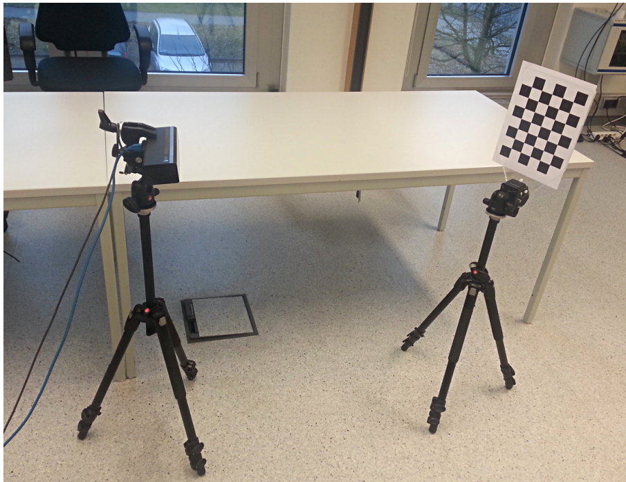
Figure 3.8 An example setup for Microsoft Kinect v2 calibration [75].
