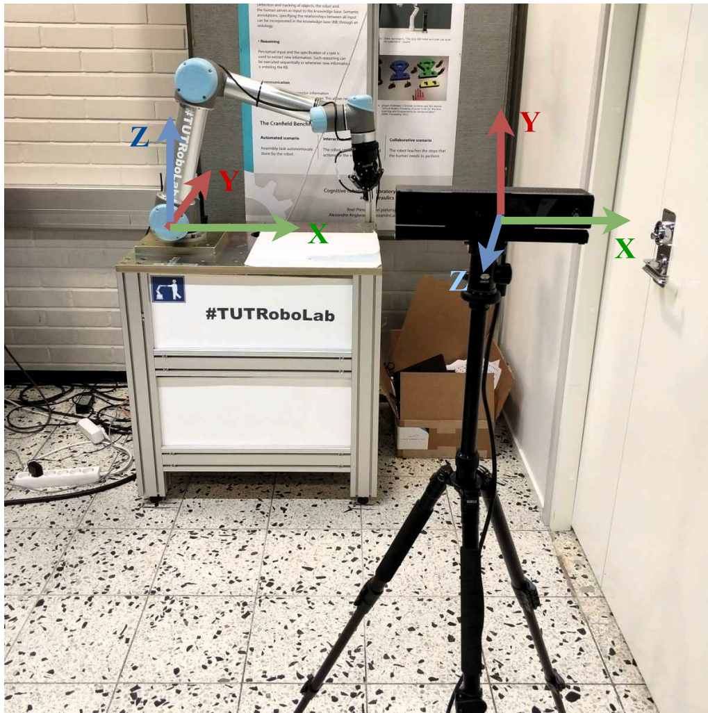
Figure 4.3 Environment of system and Cartesian coordinate system mapping between UR5 and Kinect.
