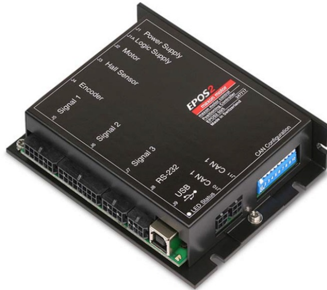
Fig. 2.2: EPOS position controller
