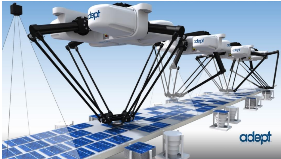
Figure 2.6 Delta robots with parallel structure [10]
