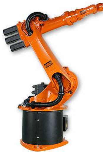
Figure 2.5 KUKA industrial robot with serial manipulator structure [23]
