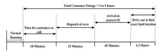
Figure 3-3: Fault Management timescale (without FLISR process)
