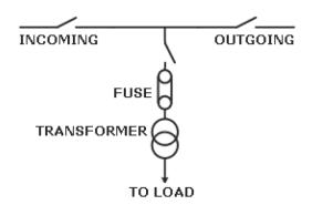
Figure 3-2: Basic RMU unit for SS
