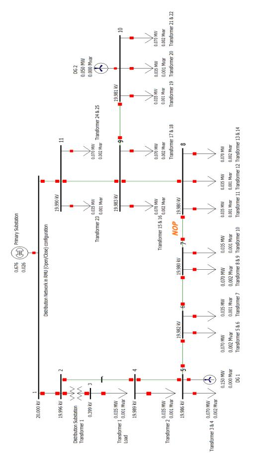
Figure 4-2: Emulated network in RMU configuration
