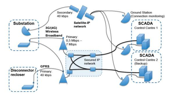
Figure 4-6: Field communication system used by Elenia (Verho, 2013)
