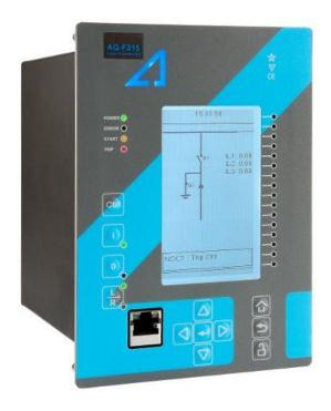
Figure 5-1: AQ-F215 feeder protection IED by Arcteq
