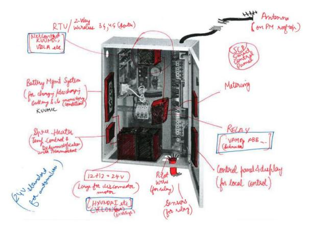
Figure 5-6: Initial sketch for SN Panel
