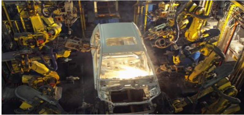
Cloud-connected welding robots on this automotive assembly line help realize the vision of Industry 4.0 by monitoring themselves for potential downtime issues and facilitating predictive maintenance. (Courtesy of FANUC America Corporation)
