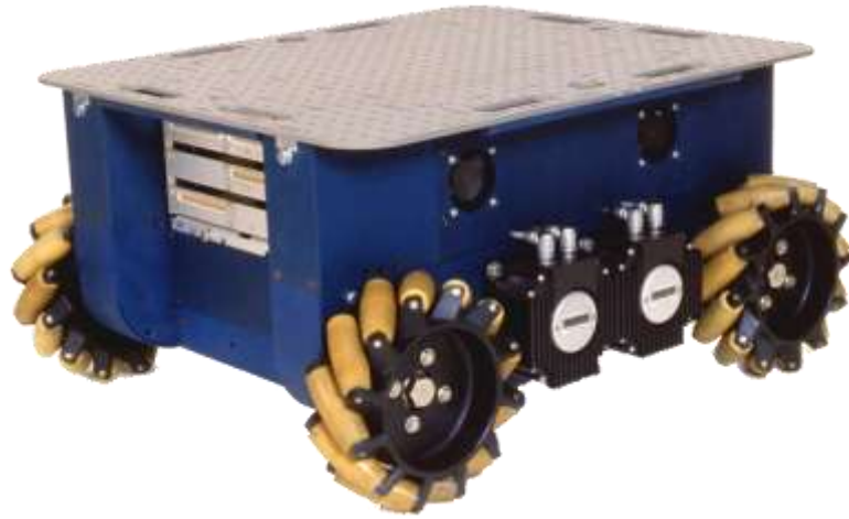
Figure 2.4. URANUS omnidirectional mobile robot
