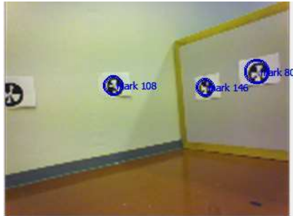
Figure 4.2. Marker detection with monitor software
