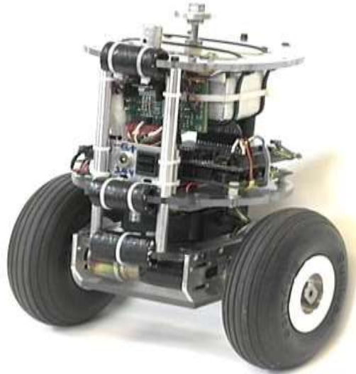
Figure 2.2. Two wheeled robot Nbot
