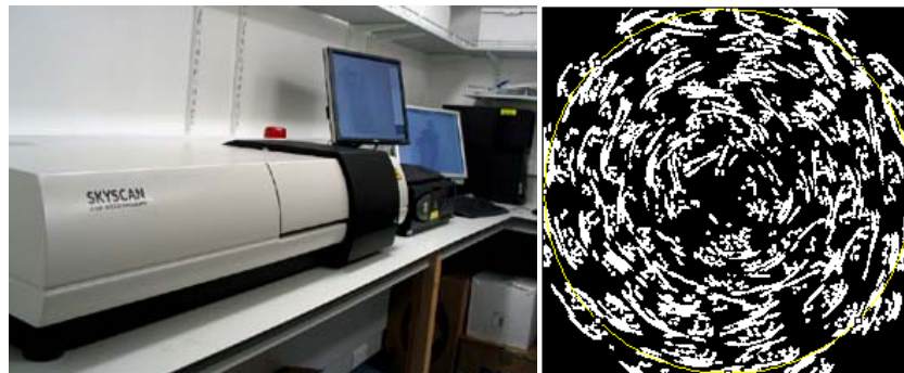
Figure 6.12. SkyScan 1072 desktop micro-CT (left) [74] and representative 2D image of P type joint scaffold using manually set threshold levels of 50 (right).
