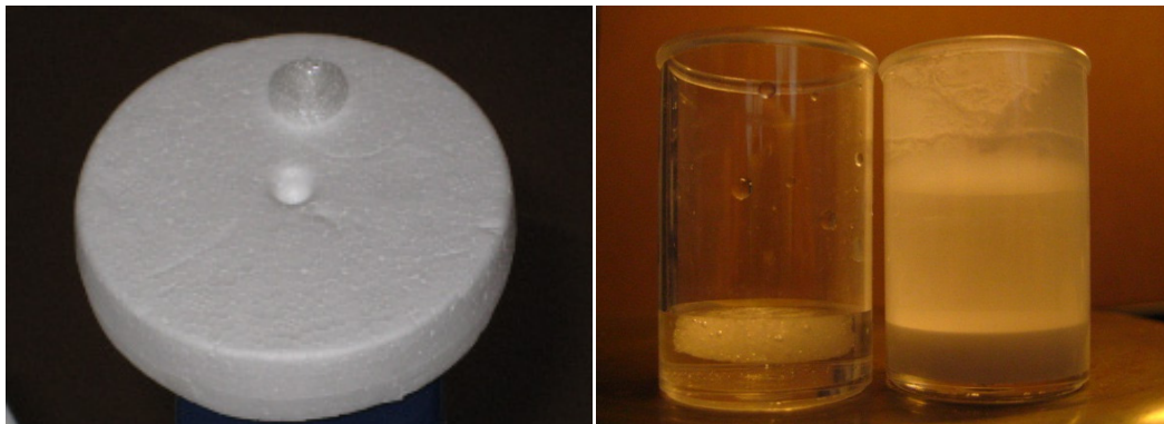
Figure 6.5. Illustration of three different imaging approaches. P(L/D)LA 96/4 scaffold was scanned in air without any contrast enhancement by putting it on a sample holder (left). Scaffolds were also scanned immersed in transparent iodine solution (left tube) and slurry of barium sulphate and water (right tube). In right tube scaffold lays on the bottom under the precipitation of BaSO_4 .
