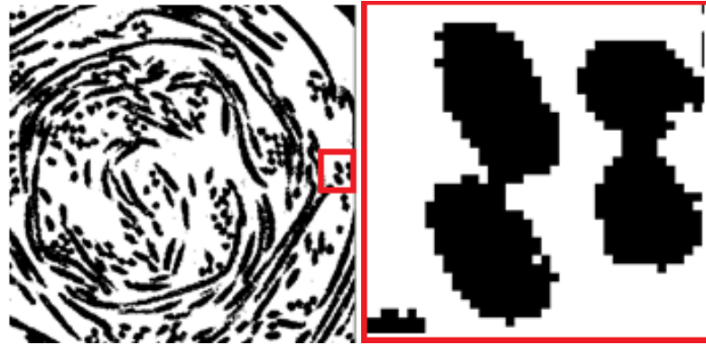
Figure 3.3. Illustration of 2D \mu CT image of P(L/D)LA 96/4 joint scaffold and a close-up of it showing the pixel map. Each pixel have own intensity value ranging between black and white. Black pixels describe polymer phase and white pixels empty regions. The image has been taken from the present study.
