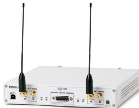
Figure 16. NI USRP2943, channel 1: transmitter, channel 2: receiver.
